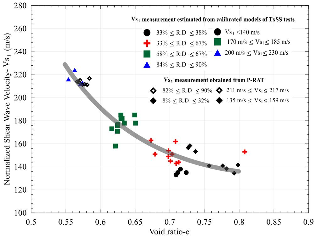
Figure 4. Variation of the shear wave velocity as a function of the void ratio from tests performed by TxSS and P-RAT
