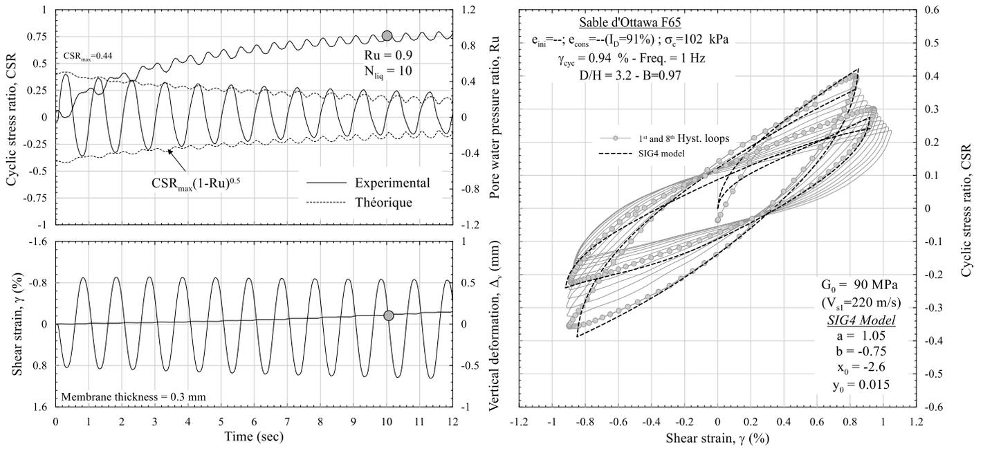
Figure 2. TxSS Records of CSR variation and pore pressure generation of Ottawa F-65
