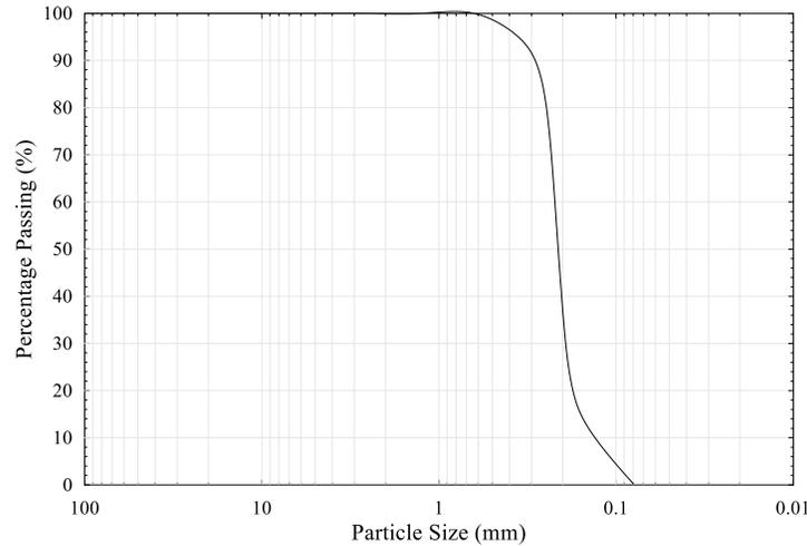
Figure 1. Grain size distribution of Ottawa F-65.
