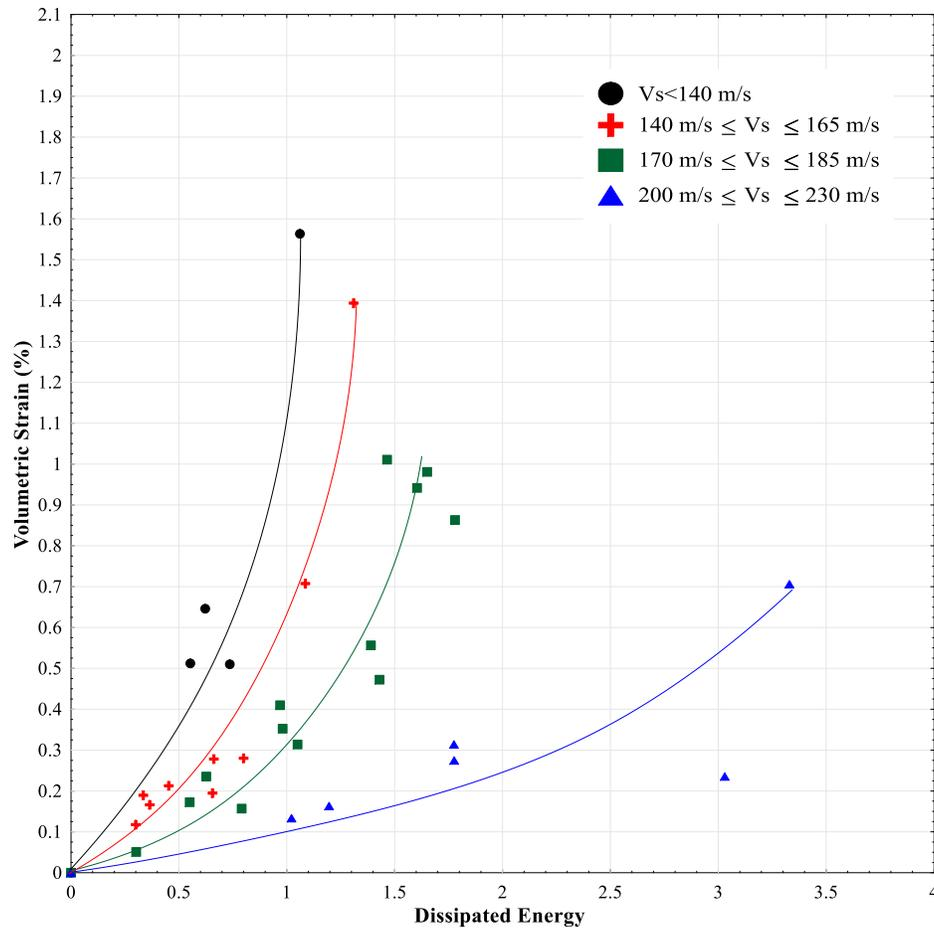
Figure 3. Variation of the volumetric strain as a function of the dissipated energy for the 34 tests.
